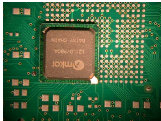
(BGA component slid into position on SSD's)
