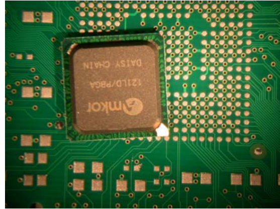
(Component placed close to final position)
